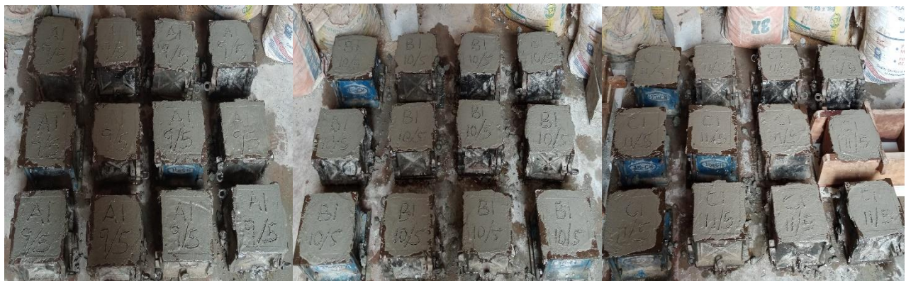
Plate 1: A Total of 36 cubes for Samples A, B and C casted in iron moulds ready for curing
